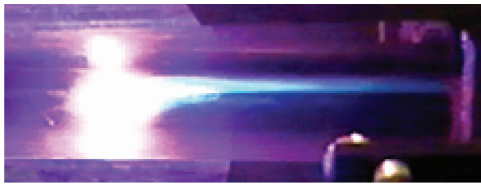
b) Aeroramp (5.4 g/s, 352 K), Freestream (5.4 atm, 592K), AC Plasma Torch (5 kWPeak, 470 SLPM Air)
