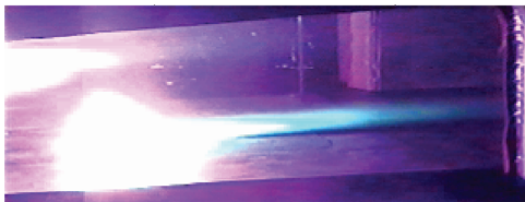
d) Aeroramp (5.4 g/s, 336 K), Freestream (5.4 atm, 586 K), DC Plasma Torch (4.0±0.1 kWDC, 40 SLPM N 2 )
